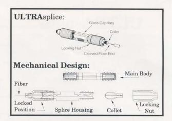
**ULTRA**splice is a high performance, low cost, easy to install, fully mechanical Fiber Optic Splice. Employing a visible glass capillary alignment member, that is pre-loaded with index matching gel, the user can inspect the fiber location during installation. The splice is tunable and reusable for most any emergency (or permanent) installation requirement(s).
